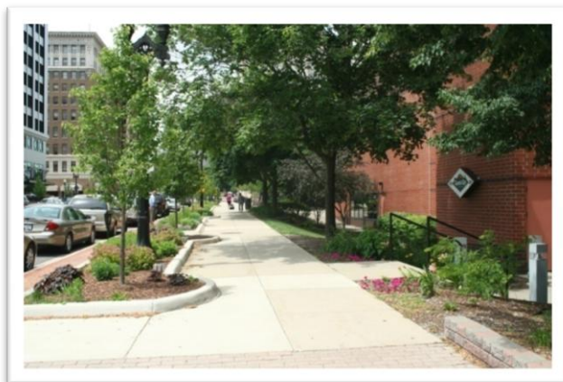
Pedestrian-friendly area on the north side of Michigan Avenue has room for roadway, metered parking, a green "buffer" zone, and wide sidewalks with attractive design features. - Lansing, MI
