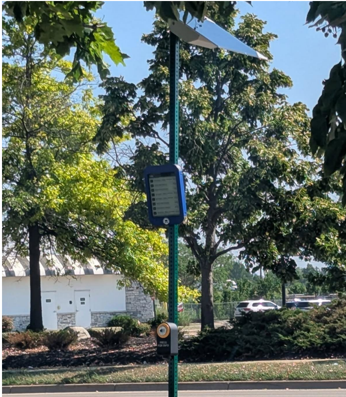
Figure 1: Example of Real Time Screen and Annunciator Currently in CATA's System
