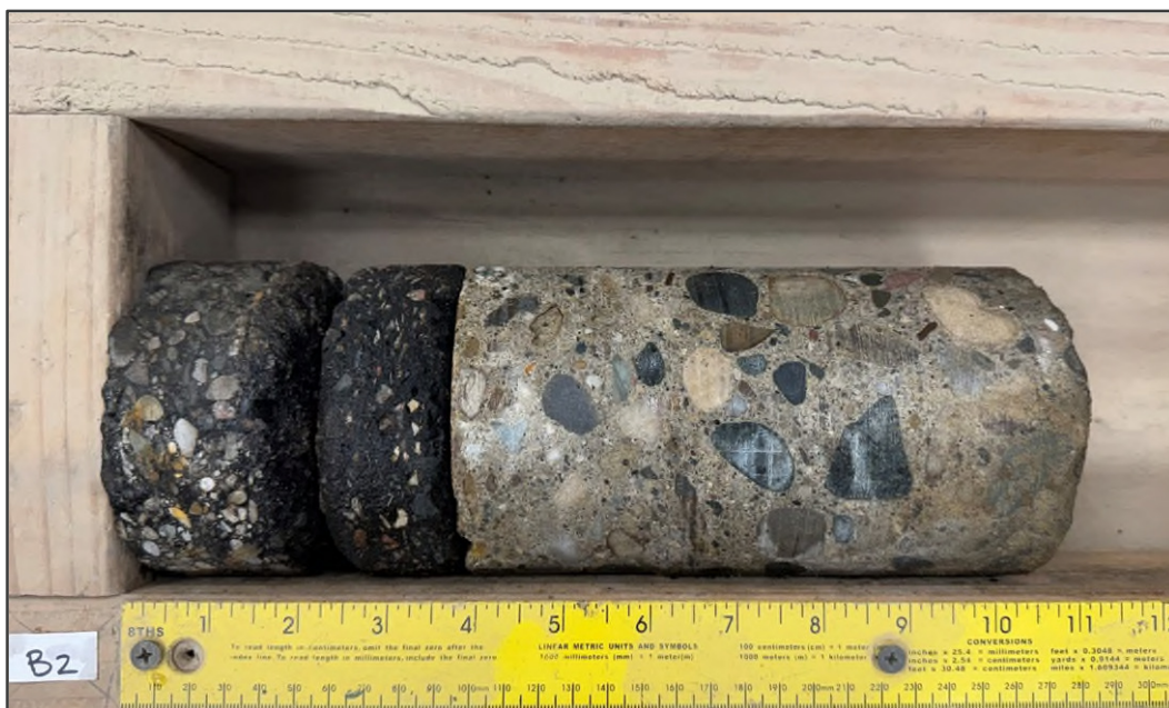
PHOTO NO. 2: Boring P2 - 4 inches of Asphalt and 7 inches of Concrete
